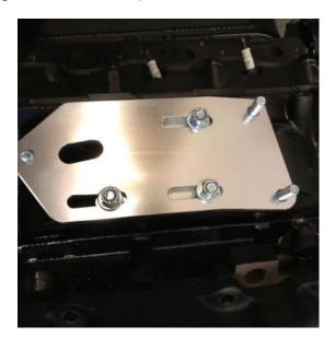
Next, mount your 1996-2004 4.6 Mustang passenger side engine mount to the outer plate. Torque all bolts to 28 ft lbs. These will fit the factory rubber or aftermarket urethane or solid engine mounts
