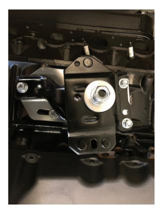
There is a large billet spacer that is installed into the 4.6 engine mount stud before placing the mounts into the factory Fox Body K-member slots. Drop engine onto cross member and install nuts on the 4.6 mounts. When you have the engine placed into the desired position, tighten the three locking nuts on the top plates to 28 ft lbs. The same process will be used for the diver side of the engine.
